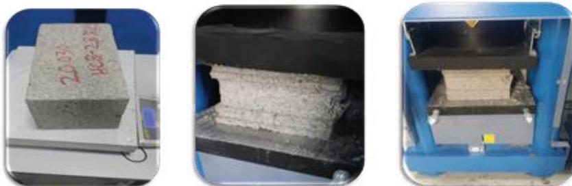
Figure 11, 12 and 13 : The Hollow Concrete Blocks after the test.
